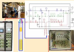
The CHOUCA device with all its pneumatic and electric components
