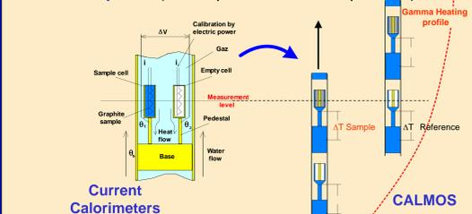
Heating measurement = K (ΔT sample - ΔT reference) = K ΔAT. K coefficient is determined from a calibration step where heat is generated using electric current
